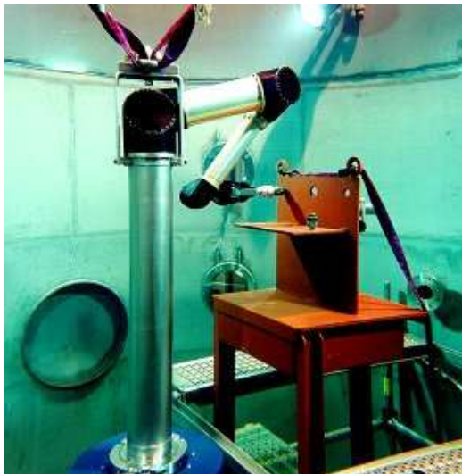
Figure 8. The slave arm of the TELBOT-manipulator during an unscrewing task
